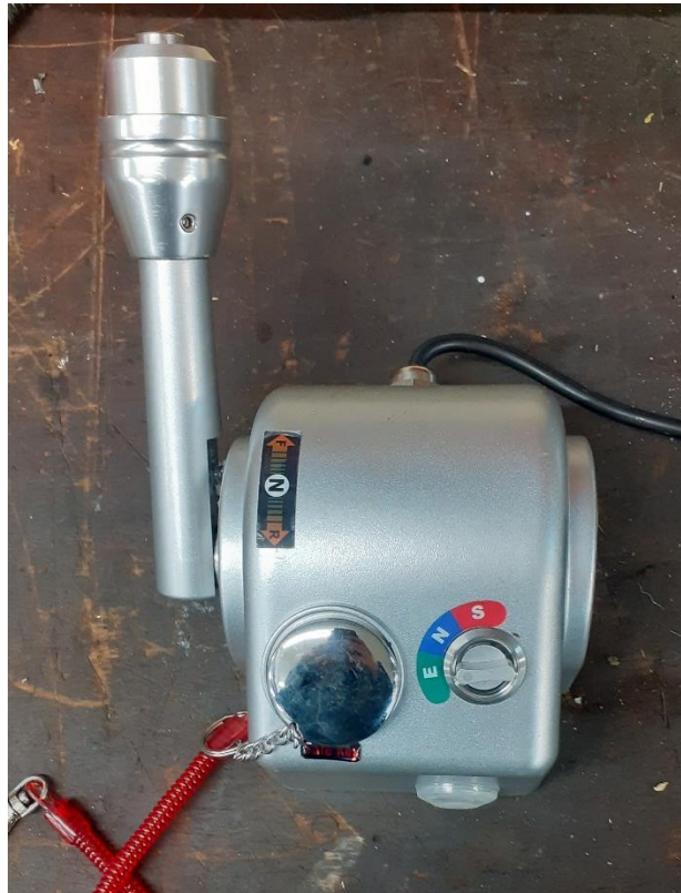
Figure 27: Speed and Direction Control Lever in forward position
