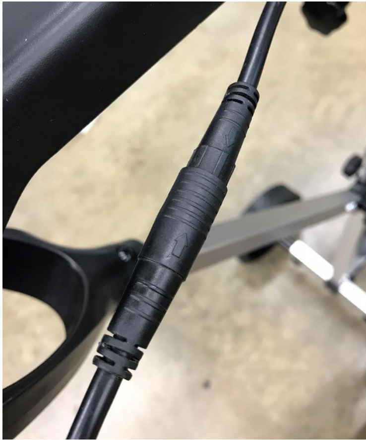
Figure 24: Control Lever connected to Outboard Motor
