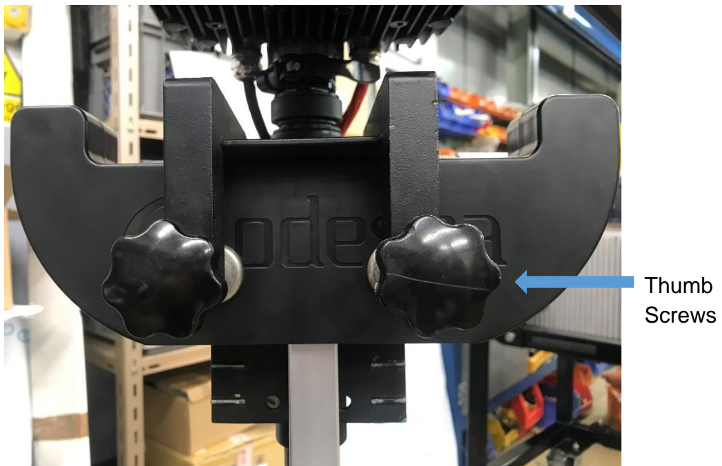
Figure 12: Fitting outboard to boat
